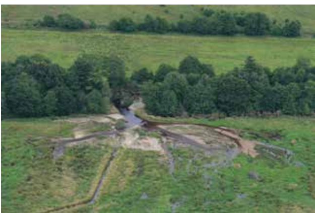
Figure 5.4 (Left) Burn of Mosset in Moray. Breaching a flood embankment has reconnected the channel to its floodplain and led to the development of complex habitat (© Scotavia Images). (Right) Setting back a flood embankment to allow the River Ribble, in Lancashire more space to spill and interact with its floodplain (© Environment Agency).
