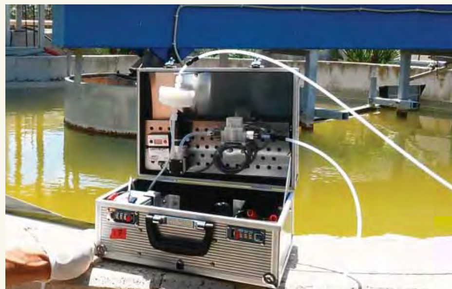
Image 21: Mariani box for wastewater collection. (Source: EC JRC, 2016)
